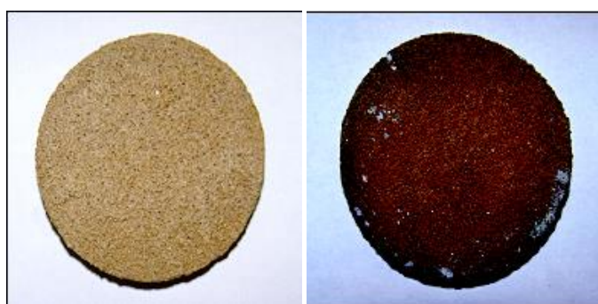
Figure 3.8. Photographs of fly ash filters before (left) and after (right) trapping gaseous caesium
