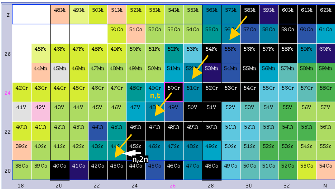
Figure 14: Depiction of the (n,t) reaction on the chart of nuclides. Four examples of isotopes selected as feasible for our experiments ( ^{58}\text{Ni} , ^{54}\text{Fe} , ^{50}\text{Cr} , ^{46}\text{Ti} ) and the possible interference with the (n,2n) channel are shown. Adapted from [21].
