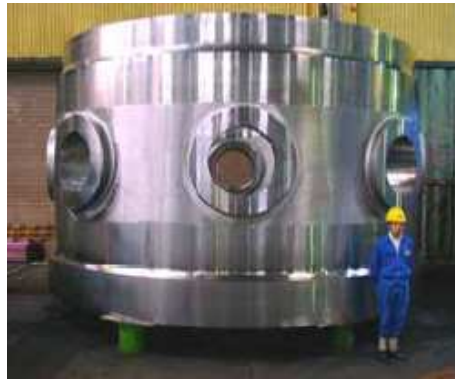
Nozzle Shell Flange
