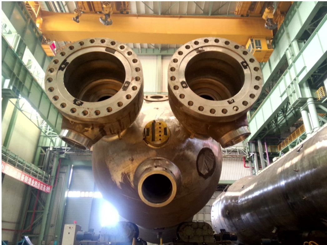
Haiyang Unit 1 – Steam generator, AP1000, China, 27 December 2014 (provided by NNSA).
