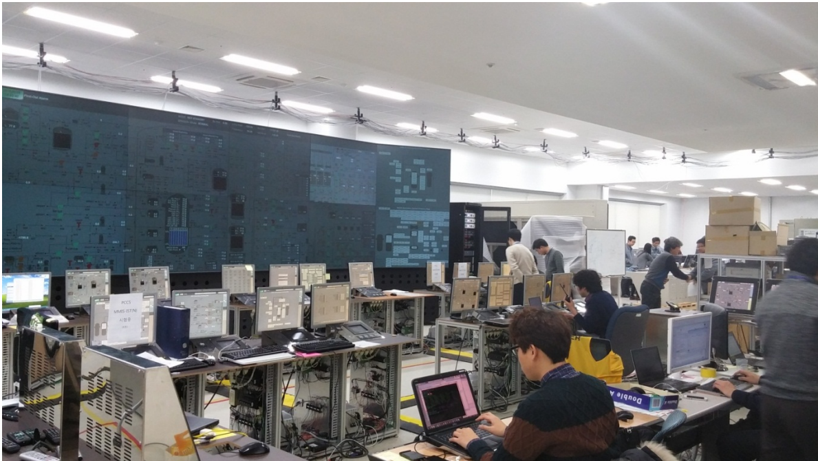
Shin Hanul – Factory integrated system test of Shin-Hanul nuclear power plant Unit 1 MMIS, APR1400, Korea, 3 April 2015 (provided by KINS).
